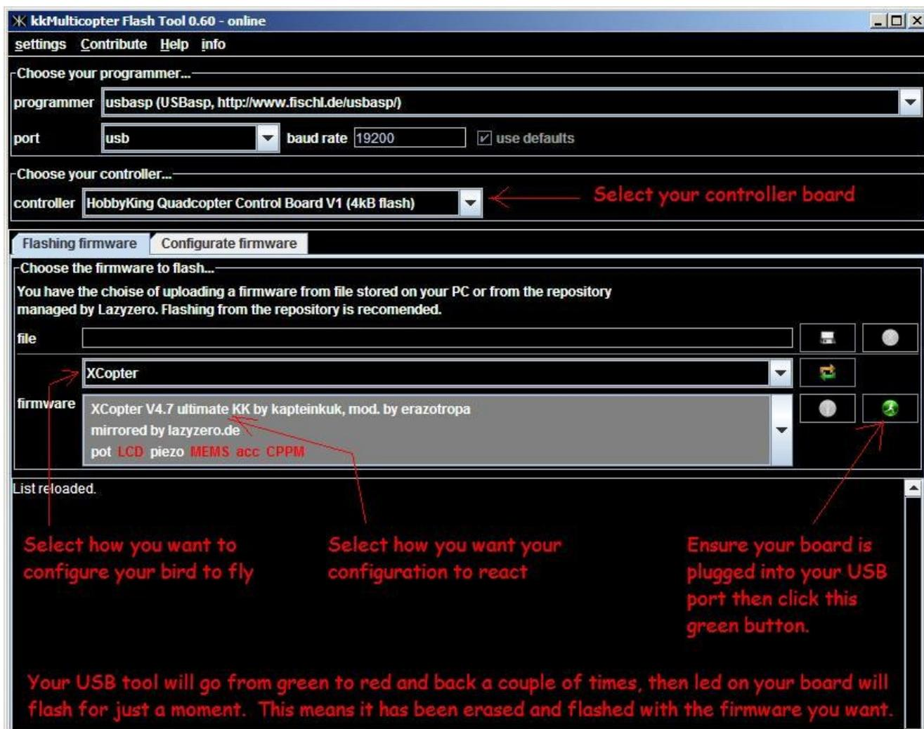
10. Your USB tool will go from green to red and back a couple of times and then the LED on your controller board will flash for a moment. This means that the board has been erased and the firmware you selected has been flashed on it.
